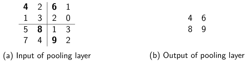
Figure 2.10.: Example of maximum pooling
